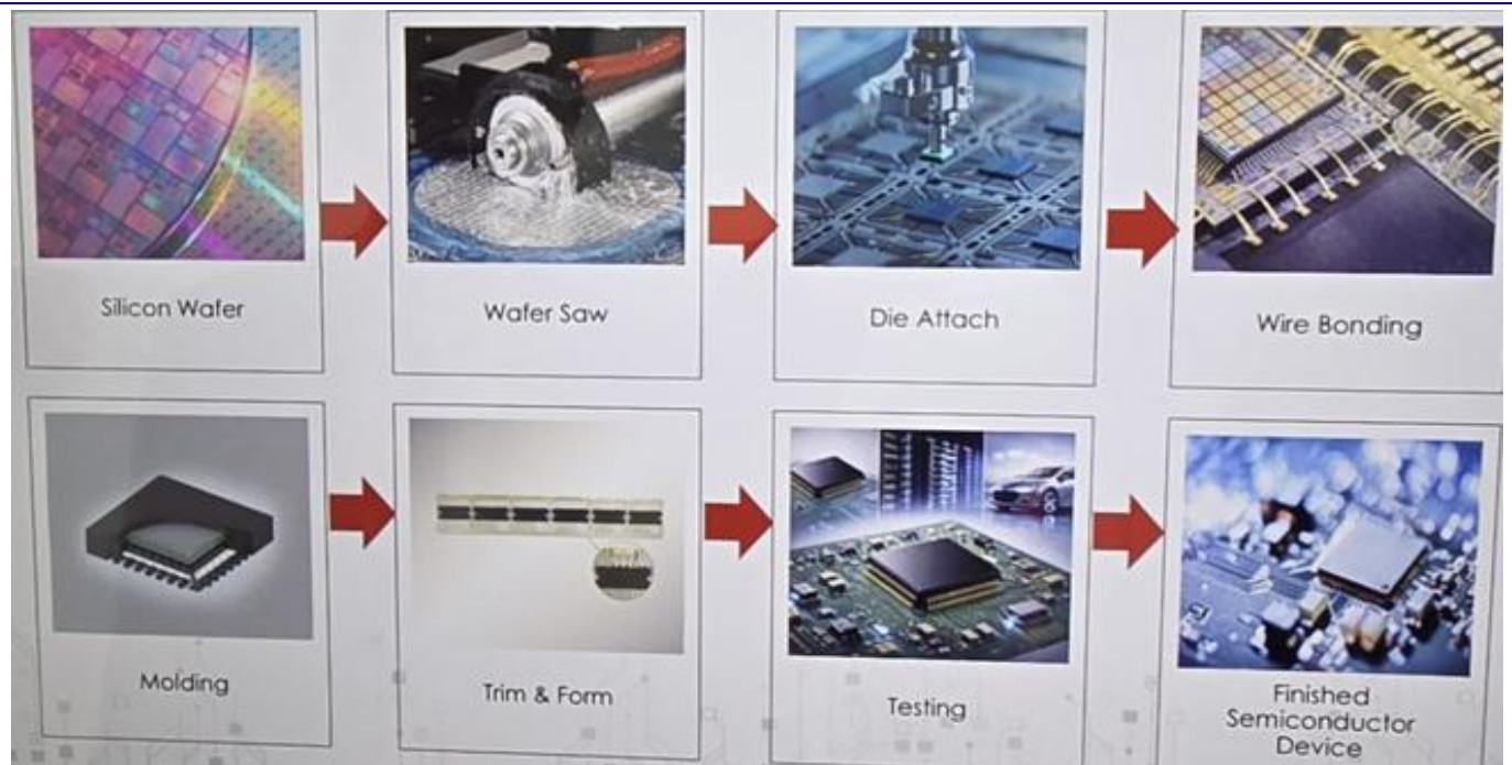
Exhibit 1: Semiconductor manufacturing process
