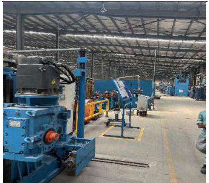
Exhibit 16: Bunching/stranding of multiple wires
