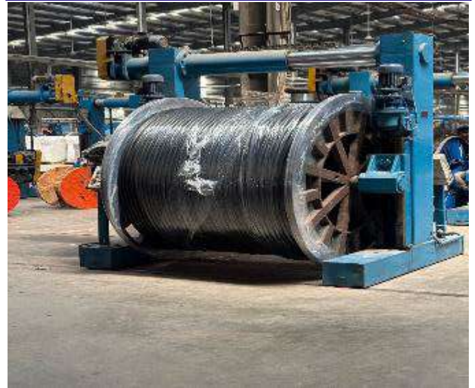
Exhibit 22: Final outer layer processed
